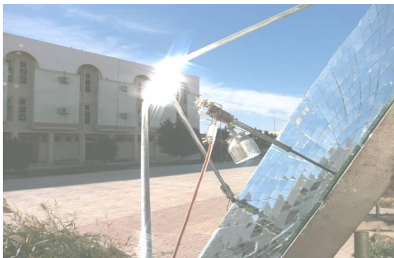
Fig. 1 A photograph of the experimental setup for the deposition of doped NiO thin films.
